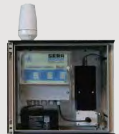
Flood warning installation with radar sensor and satellite transmission
