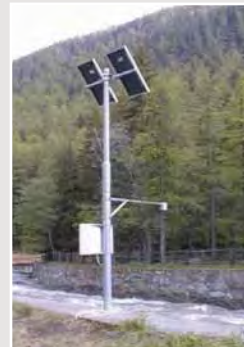
Flood warning installation with radar sensor and satellite transmission
