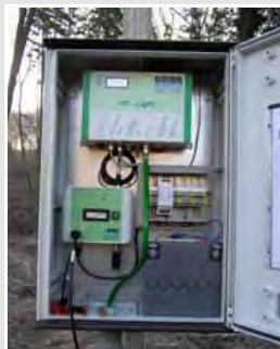
Flood measuring station with bubbler water gauge and data logger with GSM/GPRS transmission
