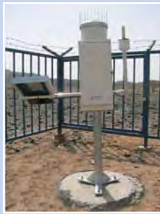
Rain station (incl. iridium modem)
