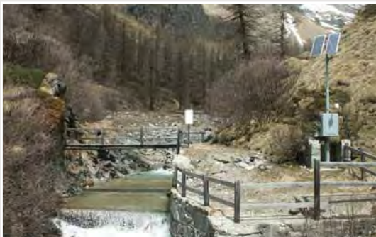
Flood warning installation with radar sensors, rain gauges and GSM/GPRS transmission
