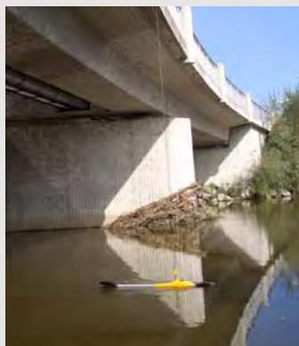
Aqua Profiler™ CW can be used with a weight for measuring from bridges and on cableway installations
